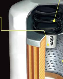
**SPIRAL PERFORATING TUBE**High structural strength to prevent the element filter from collapsing and to provide a better flow.
